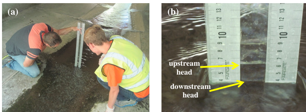
Figure 5. Measuring velocity of flow in Shotwell Brook with transparent velocity head rod (TVHR) requires the device to be held upright in stream (a). The difference in the upstream and downstream head (b) is used to calculate the velocity.
