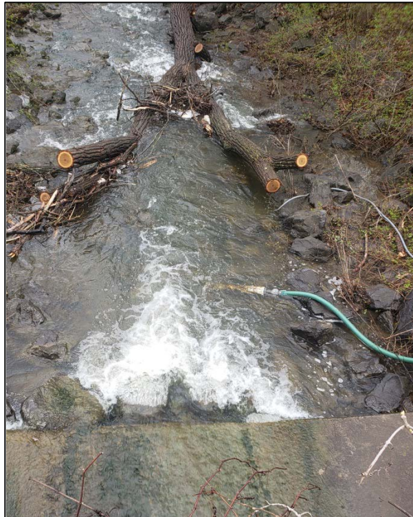
Figure 6. Position of pressure sensor (attached to gray cable) and YSI data sonde (attached to green cable) in Shotwell Brook. Photo taken in April 2019.
